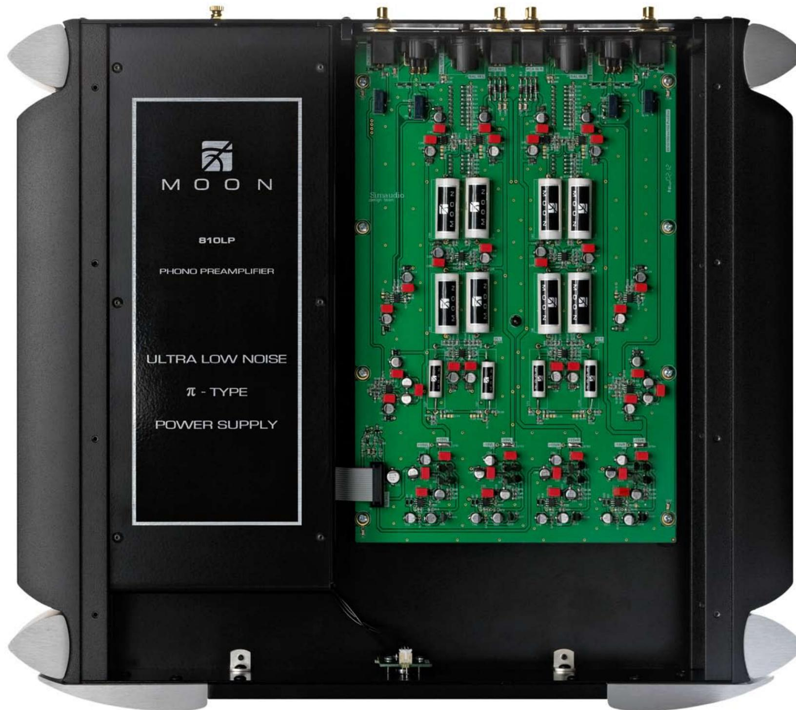
Moreover, this is a fully balanced, differential design featuring balanced XLR inputs and outputs in addition to single-ended RCA inputs and outputs. Much like a pair of headphones, a phono cartridge is a truly balanced device. Those in search of absolute maximum performance are advised to get their tonearm cable re-terminated to accommodate the Simaudio's balanced input.
