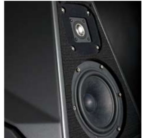
Typically Wilson: The trapezoid structure of the mid-high unit, which could be adjusted in different angles on top of the bass unit. The baffle itself is slightly inclined, the tweeter's diaphragm is a classical inverted dome type.
